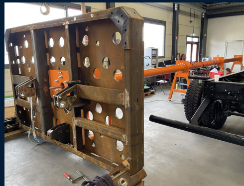
Thrust Test Frame
