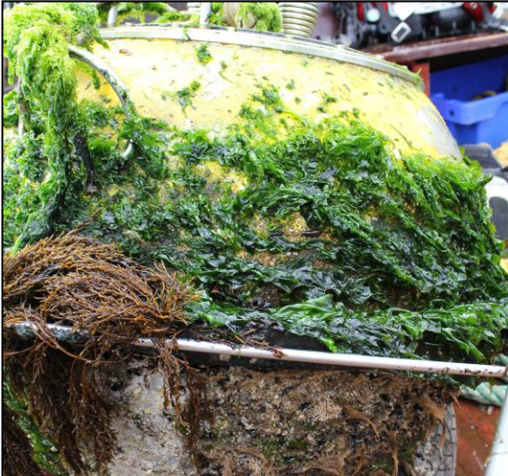
Fouling after fourteen weeks at sea.
