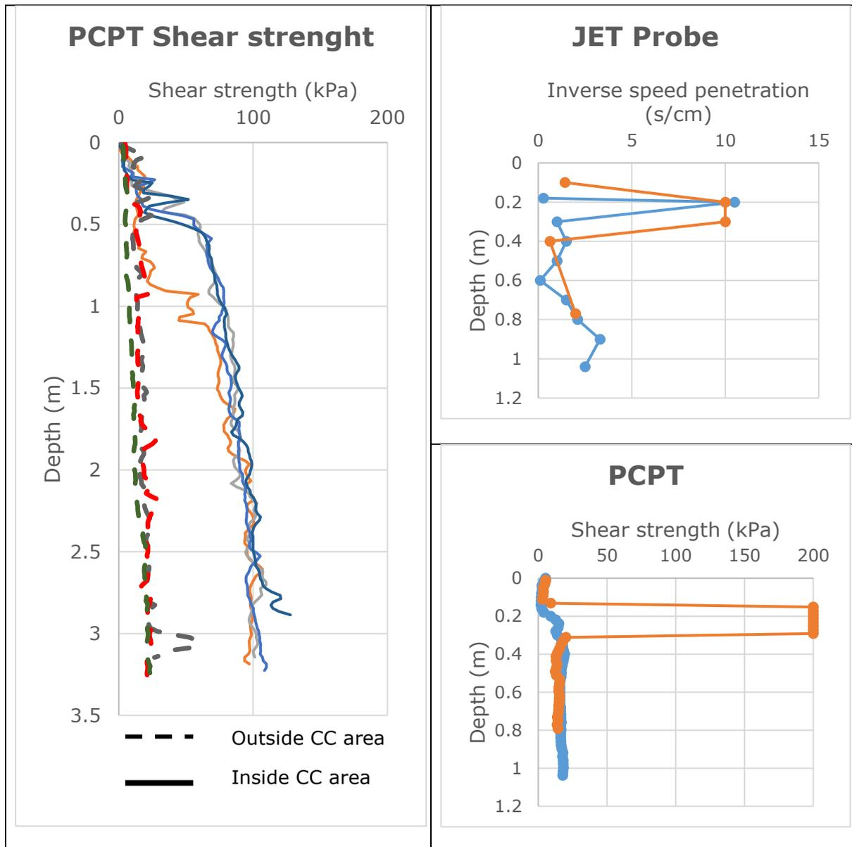
Fig. 3 – Results from PCPT shear strength analysis and jet probes inside and outside the CC outcrops.
