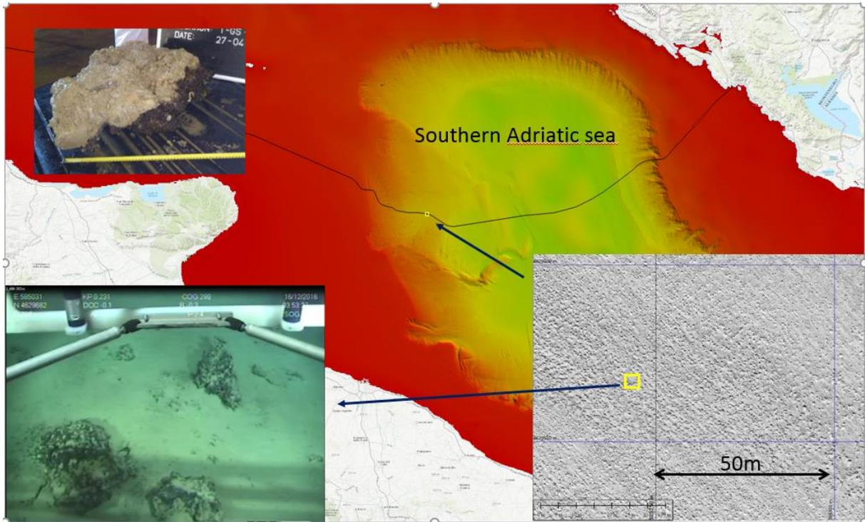
Fig. 1 – Location map with SSS mosaic on CC outcrops (right), ROV-image (bottom left) and sampled material (top left).
