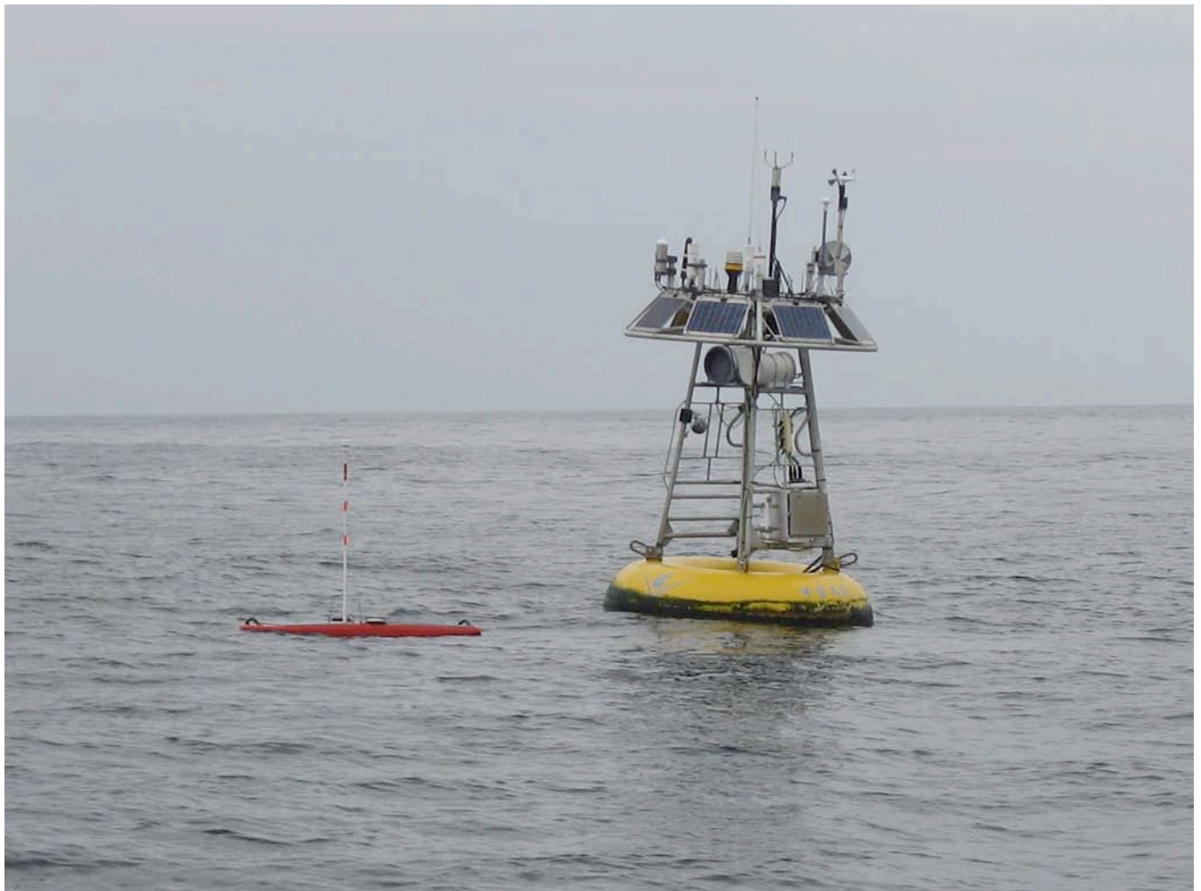
Figure 6: Wave Gliders have demonstrated station keeping superior to conventional moorings
