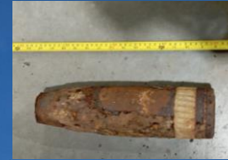
High-explosive grenade of 3.7inch (British)
