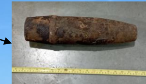
High-explosive grenade of 10.5 cm LFH (German)
