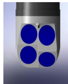
Scour Monitor head showing four transducer arrangement.
